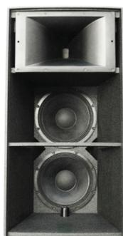
SAT 212 CX ND is a response to the rental sound industry demand for very high output and high control over output performance. Double 12" midrange transducers in short horn combined with 2" coaxial high frequency unit in large horn provides high SPL level for mid and high frequency range. It is a perfect tool for sound reinforcement at small to medium events both indoor and outdoor. It cooperates very well with TV 118 and TP 118 POL-AUDIO subwoofers.
